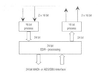
Fig. 2: Schematic representation of the 24 bit recording mode used by the D827 MCH
