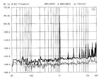
**Fig. 1**: 1 kHz, -80 dBFS: Comparison between truncation to 16 bits and 18 bit original signal (bold curve truncated to 16 bit; pointed curve 18 bit original signal).
