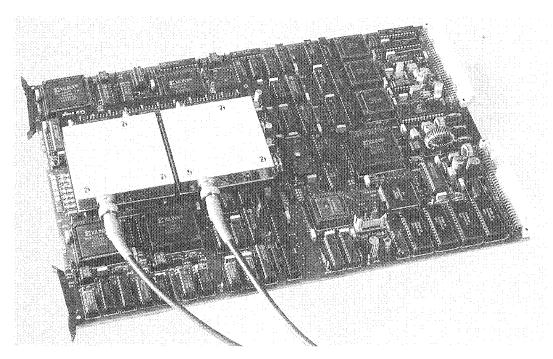
**Fig. 3:** 24 bit MADI interface board with DSP
