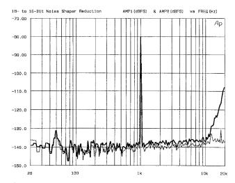
Fig. 3: Comparison between Noise Shaping and 18 bit original signal.
