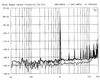
Fig. 2: 1 kHz, -80 dBFS: Comparison between truncation and noise shaping (bold curve truncated to 16 bit; pointed curve reduced to 16 bit by noise shaping).
