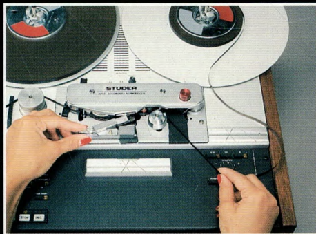
Precise tape marking, with correct tape guidance
