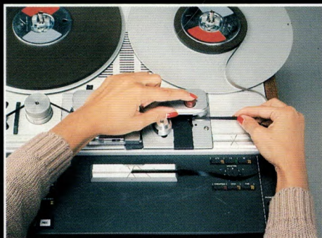
Accurate tape cutting at the correct angle for immaculate splices
