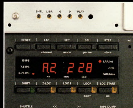
Calibration center: multifunctional keypad and display serve as the calibration instrument
