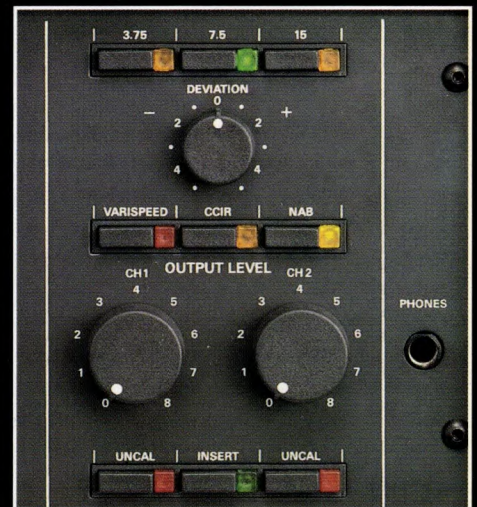
Standard features: three tape speeds, varispeed, and equalization preselection
