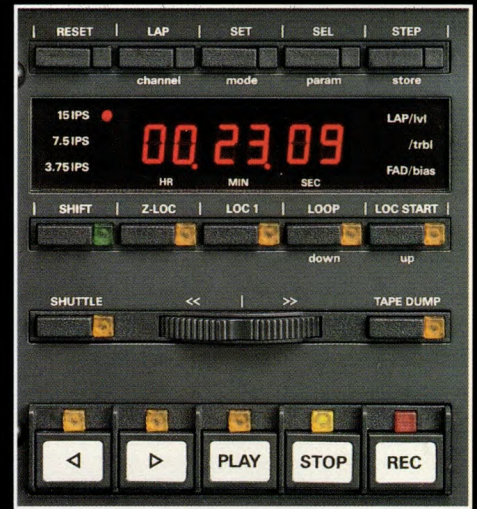
Multifunctional: Tape timer and tape transport functions
