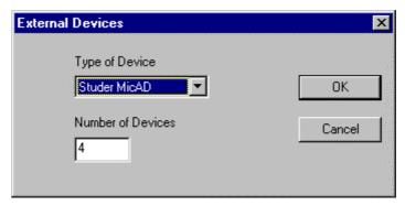
This box allows entering the number of remotely controlled devices. Currently, only the D19 MicAD can be remotely controlled from a D950. Enter the number of devices as required. The number can be higher than the actual number of connected devices.
