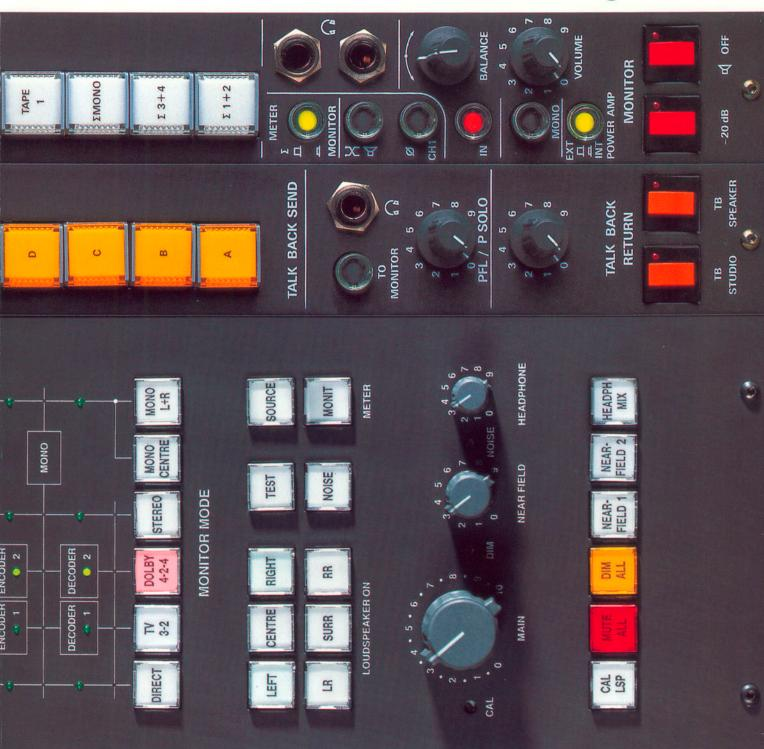
For the «Film» version a special monitor panel (bottom) is available. A source matrix allows monitoring of the mixing console information in mono to six-channels as well as monitoring of the surround channels in direct, encoded and decoded form and consequently offers quality control of the recording via the Codec links. The selected signal paths are clearly marked by LEDs. Individual speakers can be turned on and off. This panel is also able to control the near-field monitors.
