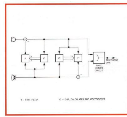
Dial tones or ringing signals can either be passed through or suppressed. The digital telephone hybrid can also be switched to 4-wire mode in which case 240 coefficients are available. For this reason this unit is suited not only for a wide range of future ISDN applications but also general echo suppression.
