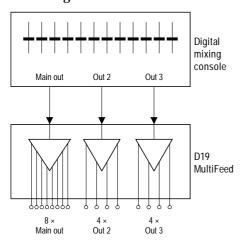
As the 16 outputs of a D19 MultiFeed can be configured in such a way that they distribute different signals, it is possible to use eight outputs for the distribution of the main output, and four of them each for two other signals, such as AUX outputs or a second master output.
