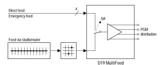
In the given example, the D19 MultiFeed will switch over to the emergency feeds in the same moment when the program feed via console and router is interrupted. This ensures that the important system output will *never* be without a signal.
