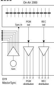
In many installations with the On-Air 2000 digital mixing console (or other digital consoles), the need arises to generate a sync signal and distribute it to some peripheral devices, such as recording machines or players.
