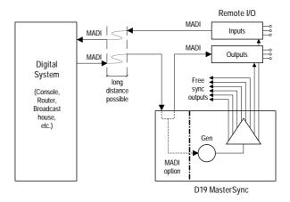
With more and more signals being transported on optical fibre links for improved immunity against signal distortion like hum, many systems have inputs and outputs located remotely. These inputs and outputs must be synchronized to the main digital system.
