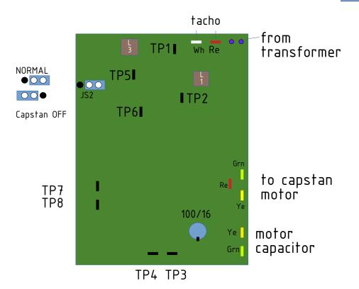
test points, connections and capacitor.
