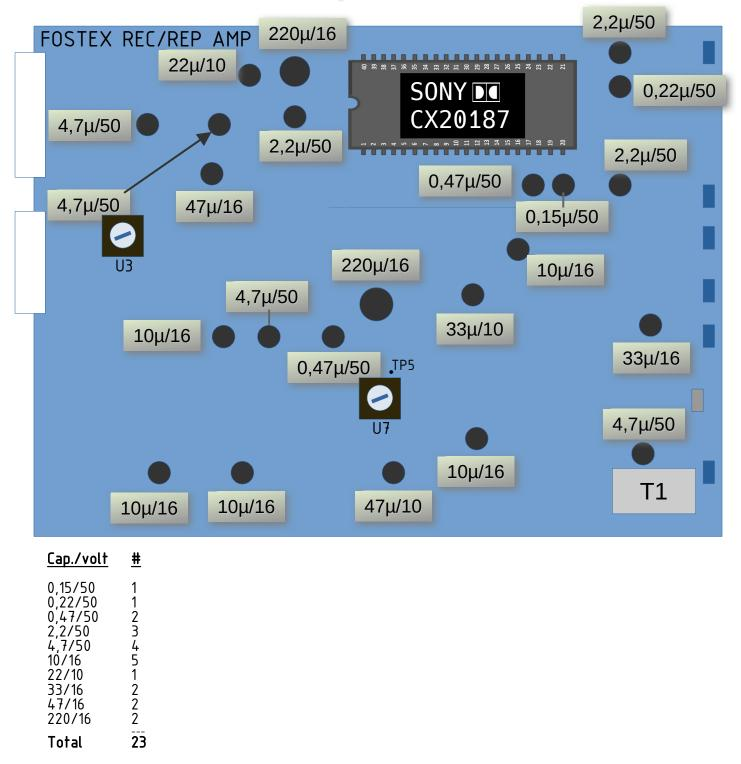
Some voltages in this <u>list</u> are higher rated to reduce the number of capacitors needed. The above diagram shows original values rast found nt | Fostex R8 | Philip van der Matten ver 3.1 | 8 jul 2024 | page 3/6
